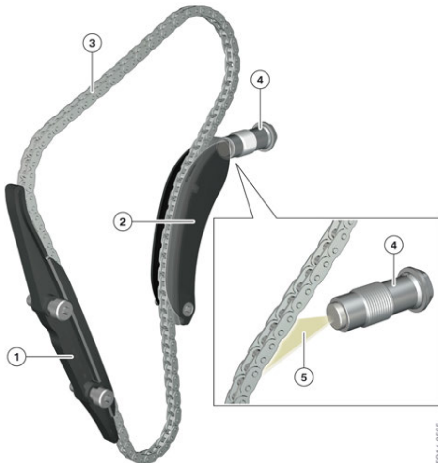
Lubrication of top chain drive, B46 engine
