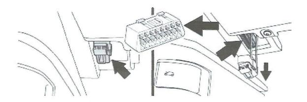
3. Plug the OBD-II cable into the OBD-II port under the dash.
