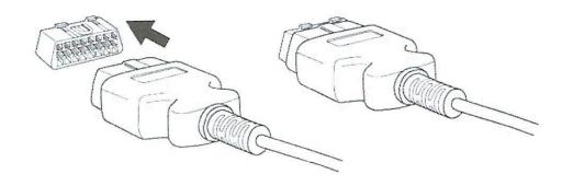
4. Connect the small end of the OBD-II cable to the 10-pin port on the bottom of the AccessPORT. At this point the AccessPORT will power up and after a few moments present the installation menu.
