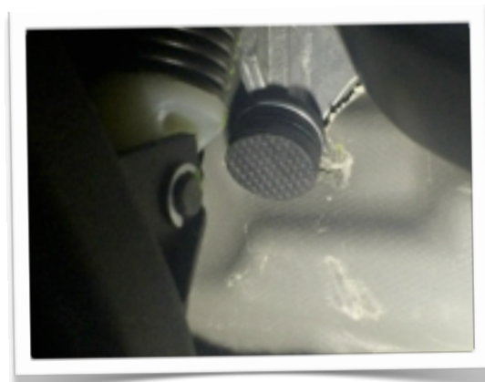
The final product: Clutch stop installed and works like a charm!
