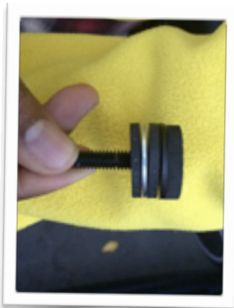
2 rubber washers and a metal washer make the perfect distance. The clutch stop comes with 3 rubber washers, so we removed one and inserted the metal
