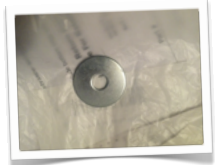
We needed the length of a 2.5 washers and this metal washer was perfect as an insertion between the rubber washers
