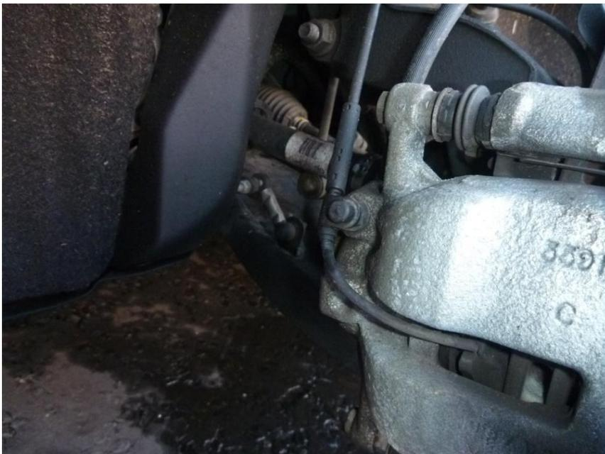
When doing the left brake, unclip the bleed nipple dust cover that (cleverly) acts as a cable guide for the brake wear sensor.
