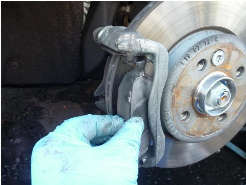
Remove the pads by sliding them away from the disc until their ears can be manoeuvred out of the slots (and the spring clips) in the calliper bracket.
