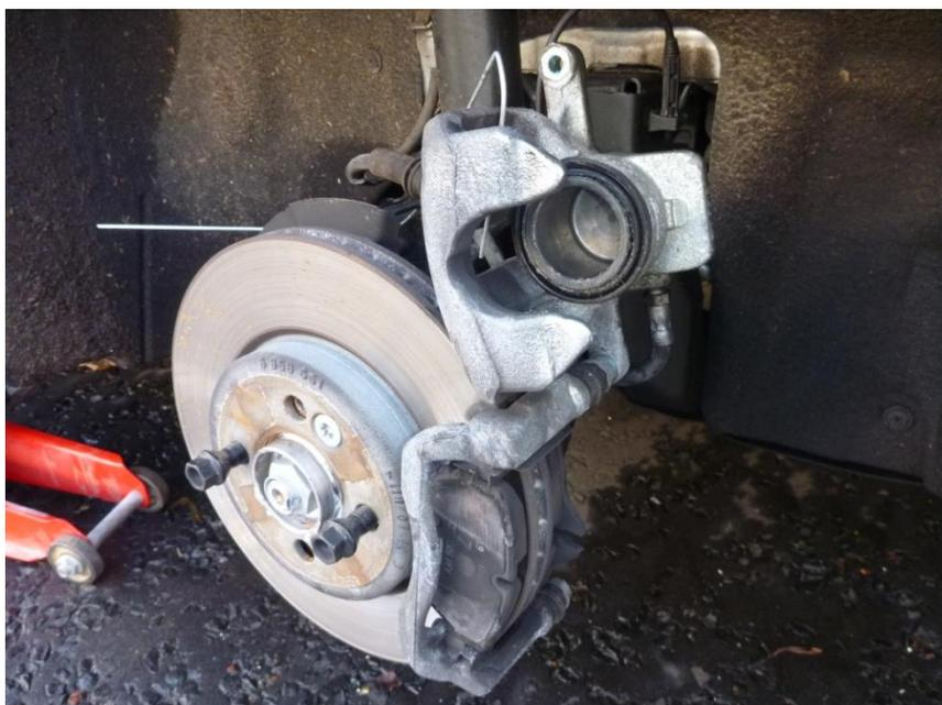
And incidentally, this is the MINI way of replacing just the pads – by undoing only the bottom guide screw and rotating the caliper up out of the way.
