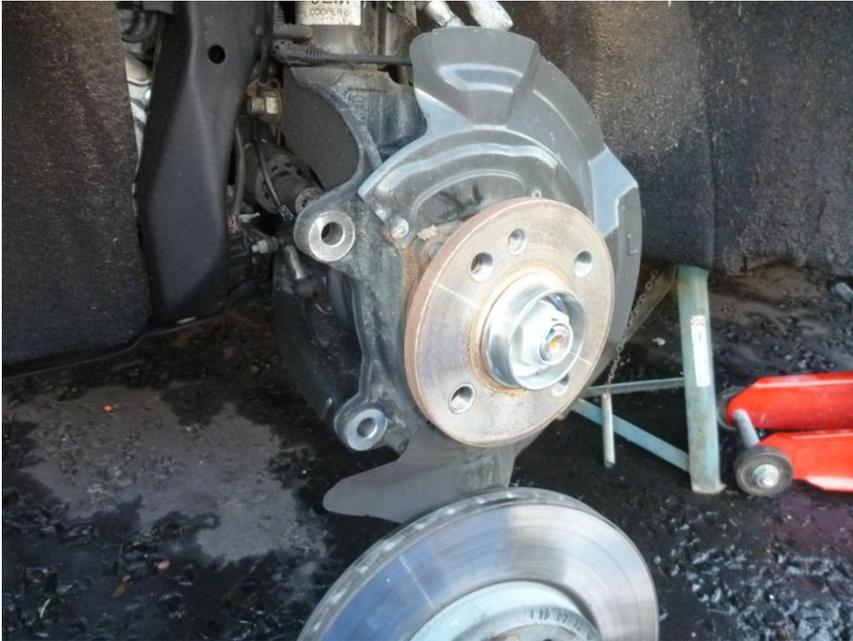
Unscrew the torx screw and a new-ish disc will fall/lift off. Discs that have been in place for a while may need some taps with a rubber mallet to loosen.
