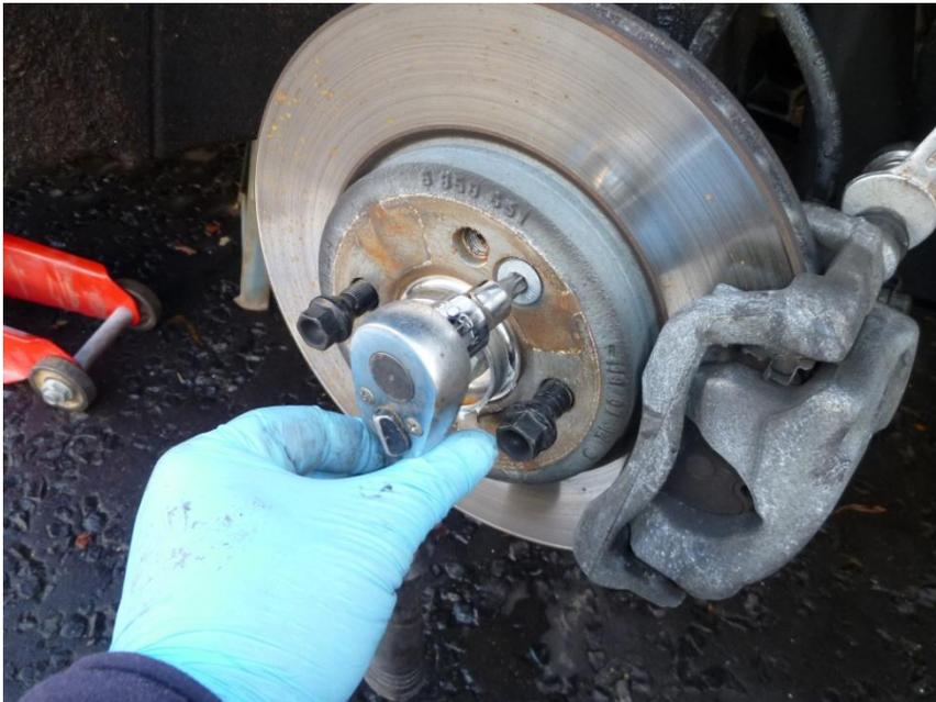
It's worth loosening the countersunk torx screw that holds the disc to the hub now – a T50 socket is required.
