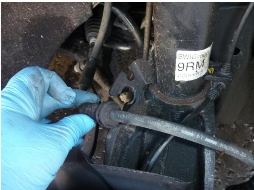
Unclip the brake hose from the strut and lift the calliper off the pads and out of the calliper bracket.
