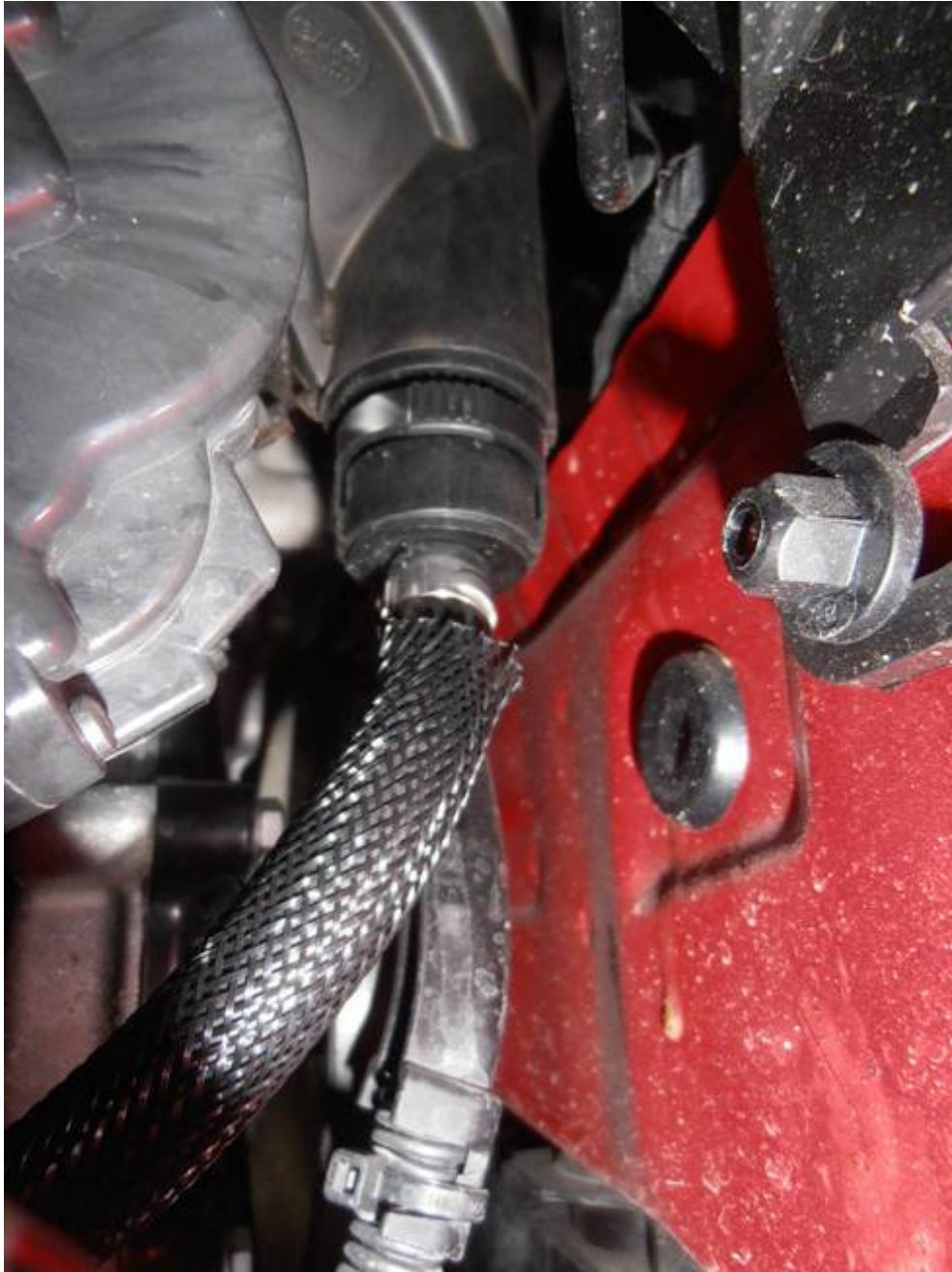
Bottom of intake at the top of this picture, this is the fitting/joint where the tube enters the intake. Picture taken with camera between firewall and engine, passenger side (location indicated on previous page)
