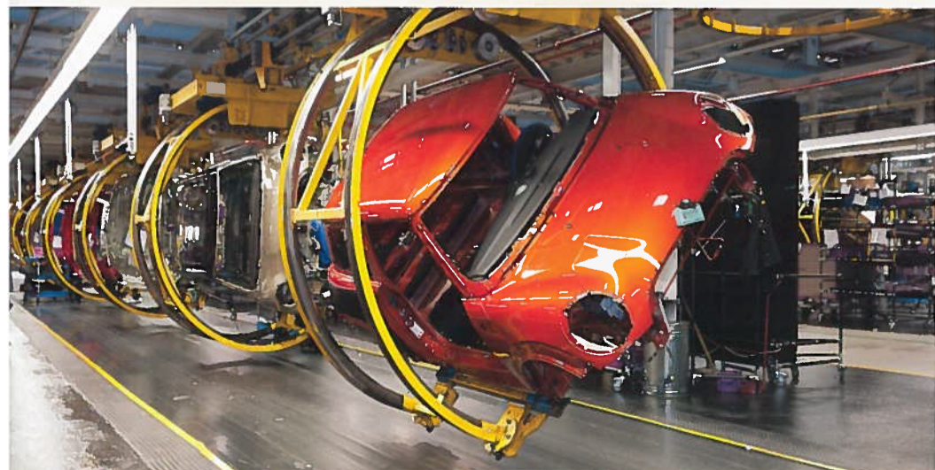
Above: Improved ergonomics: The rotary slings make it much more convenient to fit parts such as brake pipes underneath the car body. Right: The engine marriage is now a highly automated process. Associates carry out quality controls.
