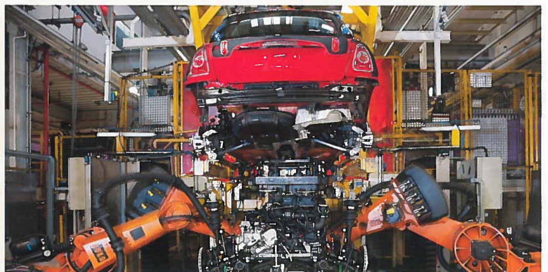
Above: Improved ergonomics: The rotary slings make it much more convenient to fit parts such as brake pipes underneath the car body. Right: The engine marriage is now a highly automated process. Associates carry out quality controls.
