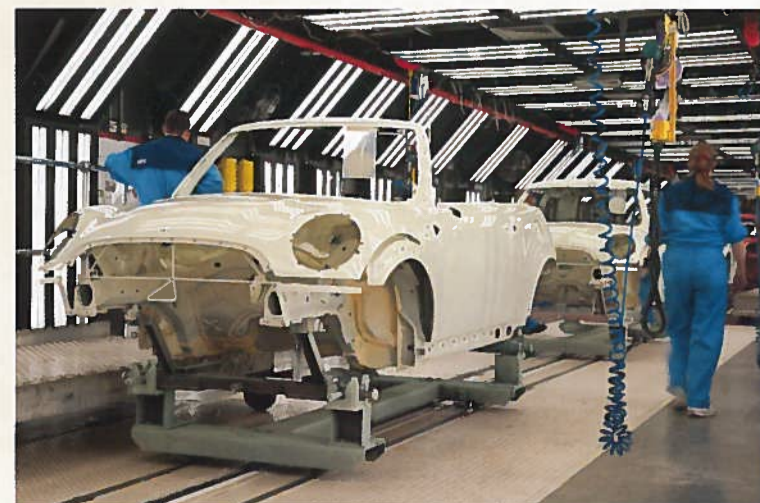
State-of-the-art technology in the current paint shop: MINI body shells leaving the oven (above left), being sprayed in the paint booths (above right and below) and on the polishing line (below right).
