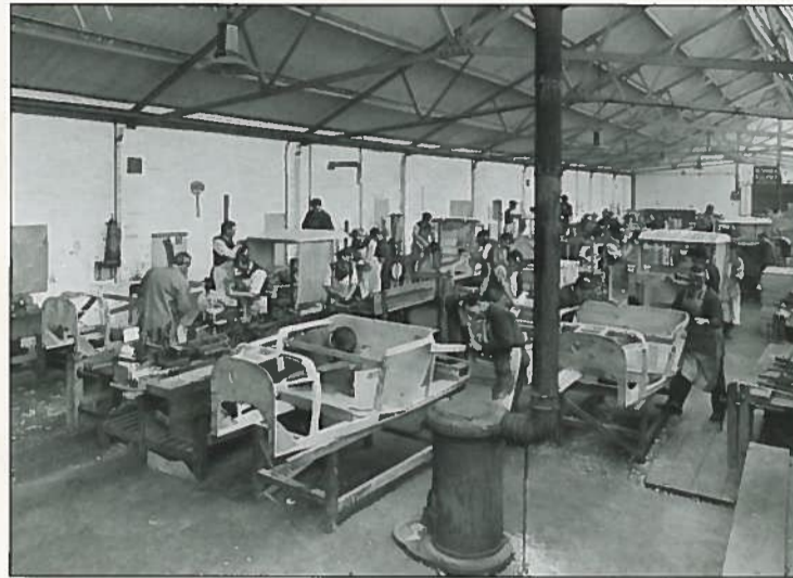
Workers finish off wooden body frames for the panelling. In the sheet metal department, the wooden bodies were panelled with metal sheets (1925).
