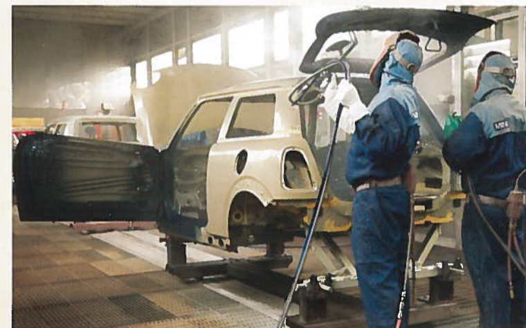
State-of-the-art technology in the current paint shop: MINI body shells leaving the oven (above left), being sprayed in the paint booths (above right and below) and on the polishing line (below right).
