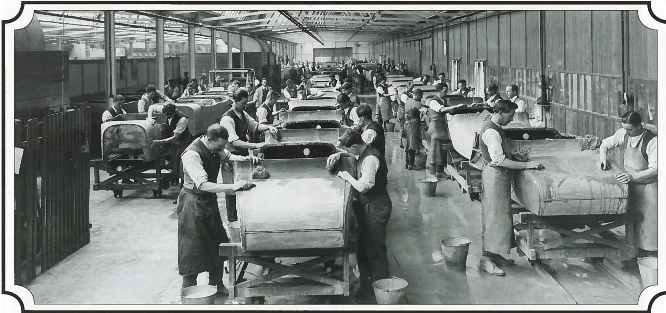
Workers had to rub down the body by hand before the painting began (1925).
