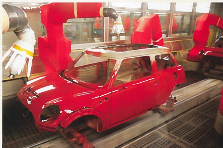
State-of-the-art technology in the current paint shop: MINI body shells leaving the oven (above left), being sprayed in the paint booths (above right and below) and on the polishing line (below right).
