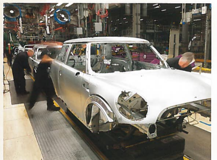
Robots weld and fix parts to the body as MINIs are moved through on a conveyor belt (left). Associates carry out quality checks on the finish line.
