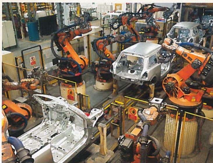
Robots weld and fix parts to the body as MINIs are moved through on a conveyor belt (left). Associates carry out quality checks on the finish line.
