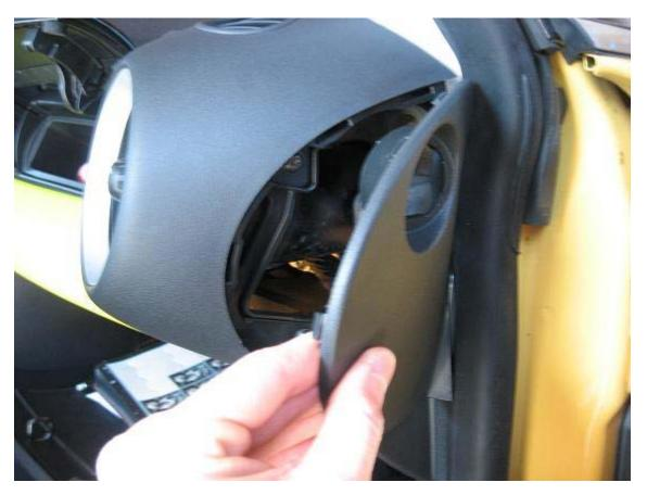
**2)** Then you are going to Pull down the window weather strip on the "A" Pillar slightly to allow access to "A" pillar trim.
