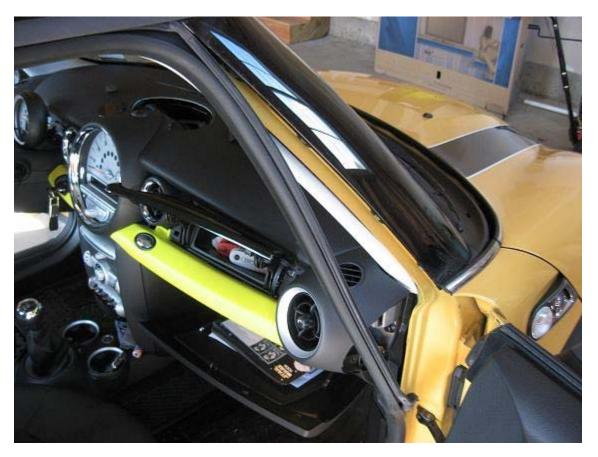
3) Then With a small screwdriver, pull out the "airbag" cover, pry lightly from the side closest to the rear of the car. Then remove the screw behind the cover. Then you will pull the pillar covers from the
