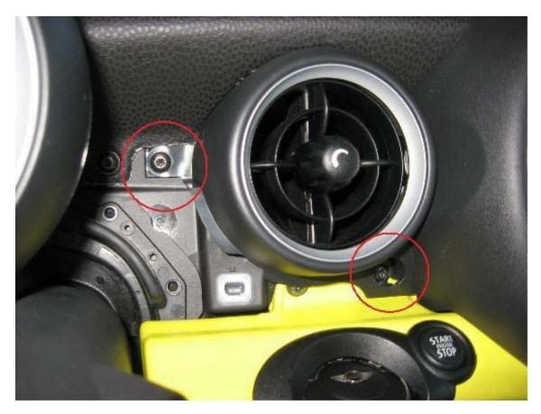
Next, you will need to remove two screws that secure the top of the speedometer trim In the two corners of the top vent in the center of the dash, there are covers that look like vent slats. (circled in red, they go where the red arrow is. You will have to snap them out. Then the screws are deep and at an angle but come out with the same size torx bit as the ones for the vents. (three photos below)
