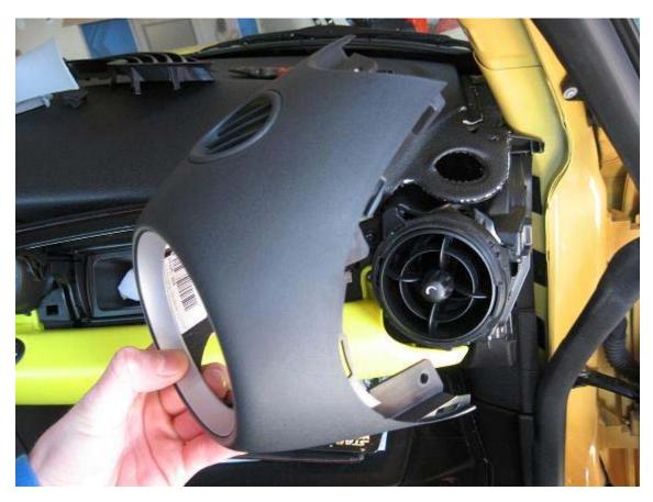
FYI: All the screws are the same except the one that hold's the "A" pillar trim in. It has a washer type on it. :)
