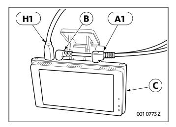
Connect branch **A1**, GPS antenna **B** and branch **H1** (optional) to front camera **C**.
